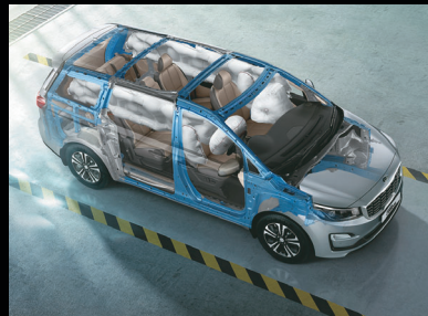
Six Airbags Our multi-directional safety package includes driver, passenger, side, and curtain airbags.
