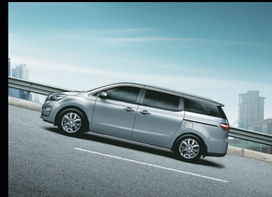
Hill Start Assist Control Hill Start Assist Control prevents the vehicle from rolling back during uphill climb from a static position.
