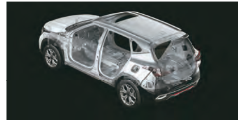
73% HIGH STRENGTH STEEL STRUCTURE Kia Seltos structure uses high-strength steel and adhesives for comprehensive safety.
